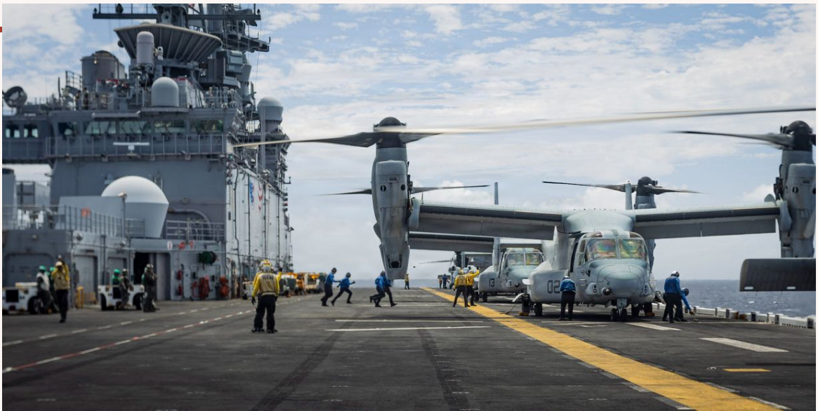
U.S. SAILORS, ASSIGNED TO THE IWO JIMA AMPHIBIOUS READY GROUP, REMOVE CHOCKS AND CHAINS ON AN MV-22B OSPREY TILTROTOR AIRCRAFT ON THE FLIGHT DECK OF WASP-CLASS AMPHIBIOUS ASSAULT SHIP USS IWO JIMA (LHD 7) WHILE UNDERWAY IN THE CARIBBEAN SEA, MAY 1, 2026 | SOURCE: U.S. SOUTHCOM.
