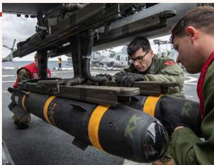
U.S. MARINES INSTALL AGM-114 HELLFIRE MISSILES ONTO AN AH-1Z VIPER ATTACK HELICOPTER | SOURCE: DVIDSHUB
